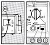
Connect the projector to the mains supply with the lead (13). Push the mains switch (26) down — this switches on the projector.
