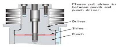
Special forming shim set(sells separately) has 5 pieces shims. Thickness is t=0.4, 0.5, 0.6, 0.7, 0.8mm It can be adjusted by those combination from 0.4mm to 2.6mm 0.1mm step.
