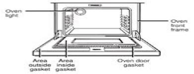
3. Clean spatters or spills on the oven front frame, and the oven door outside the gasket with a dampened cloth. The oven front frame and the oven door outside the gasket do not get cleaned by the self-clean cycle. On these areas use detergent and hot water or a soapfilled steel wool pad. Rinse well with a vinegar and water solution. This will help prevent a brown residue from forming when the oven is heated. Buff these areas with a dry cloth. Do not clean the gasket.
