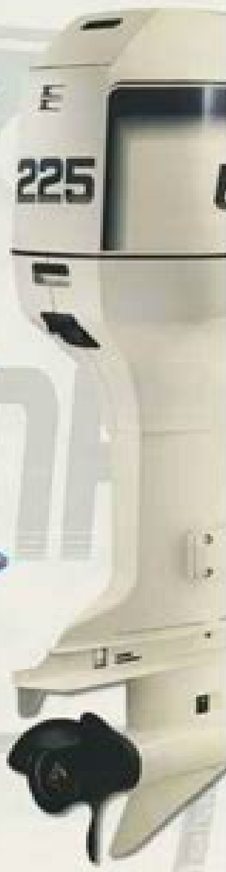
Our closed-deck powerhead, finger port cylinder sleeves and Power Path™ induction system are all designed to maximize both power and fuel economy.
