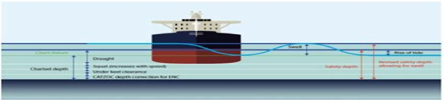
The ECDIS safety settings depended on the navigation area and depth of waters, as follows:
