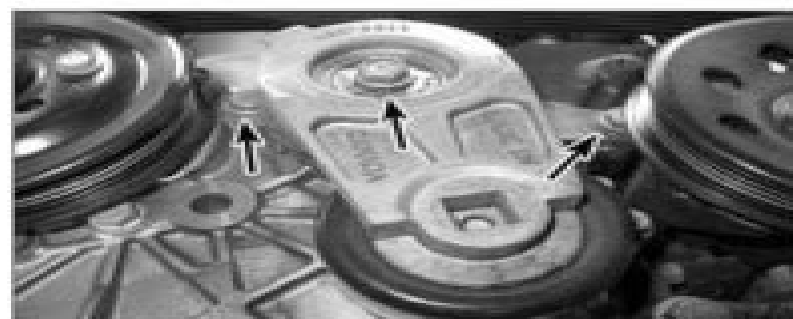
24.25 Typical V6 tensioner mounting fastener locations
