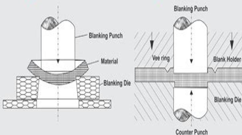
Die Clearance 5% Sheet Thickness
