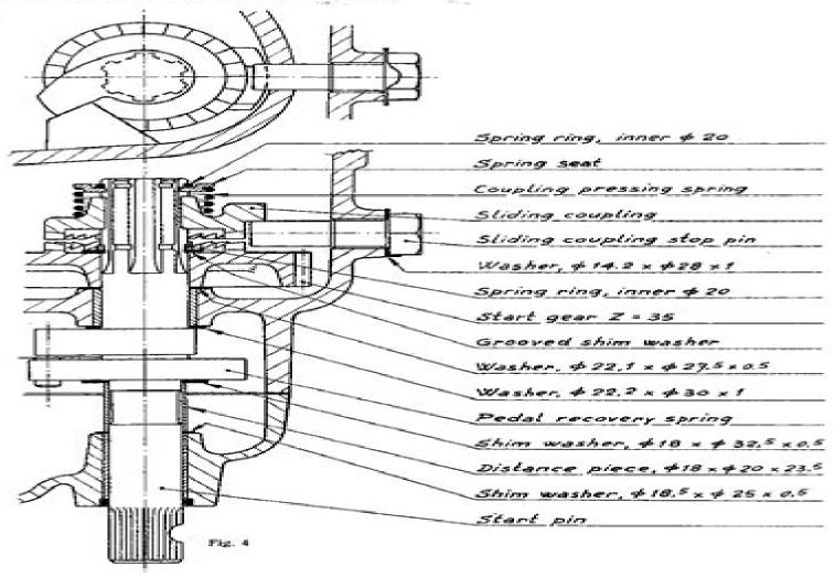
Assembly of the Flywheel-magneto, Kick-Starter and Clutch Housing (page 81)
