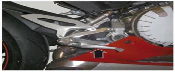
Disassembly of the fairing To disassemble the left-hand side fairing, loosen the screws (8) retaining the upper half-fairing to the lower one, and remove washers (9).
