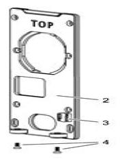
The product consists of the terminal housing (1) and the mounting plate (2).
