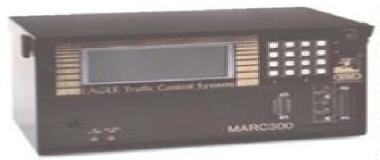
The MARC300 series controllers are the coordinating masters in Siemens ITS's closed-loop traffic control system. As a master controller, the MARC combines system management control, monitoring, and data collection capabilities for up to thirty-two (32) intersections. One MARC controller can control and supervise the Traffic Program Selection for two (2) independent groups.
